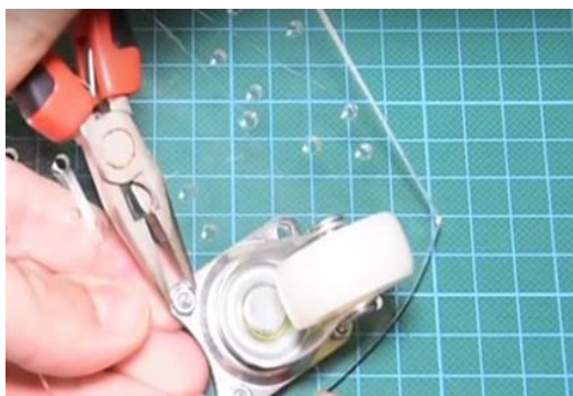
Figure 11. Attach the front wheel
